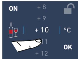
**2)** Scroll the values up or down to select the desired temperature (in the case of the cantina compartment the temperature can be set from +4 °C to +18 °C)
