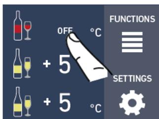
**1)** Home screen. To turn back on an off compartment, touch the **OFF** compartment next to it.
