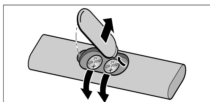
**3 Correctly insert the new batteries (3 V CR 2032).**
