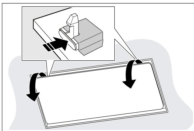
**2 Open the filter cover fully and without pulling on it.**
